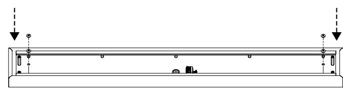
3) Drill fixing holes into ceiling and screw into place. Use x4 M6 bonded washers supplied to ensure IP seal.
