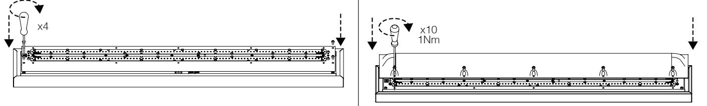
8) Screw Lens to Body with M6 x 16 screws and washers
