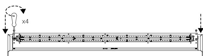
7) Place Gear tray into body and screw into place with M6 x 12 screws
