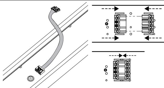
5) Connect flying lead from body into gear tray.
