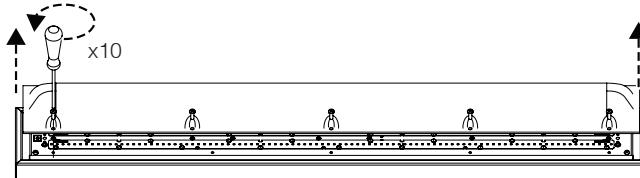
1) Unscrew and remove lens, setting aside M6 x 16 screws and washers
